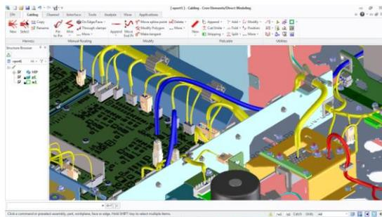
SpaceCable provides standard checks to verify that wires, splices and cables have been properly defined.
